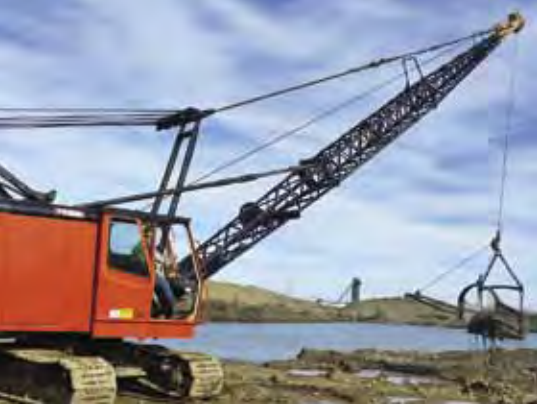
Member Dwite Forbush operates a Northwest 41 dragline with a 4-cylinder Murphy diesel engine.
