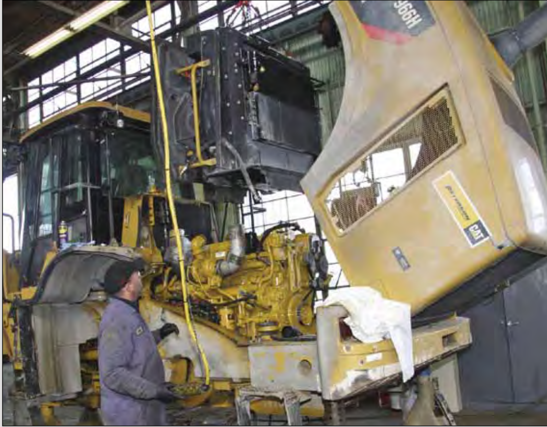
Trainee Eddie Thoits works on a coolant pack for a 966. He used to work on Wall Street.
