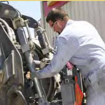
Working Foreman Justin Walker replaces the hydraulic couplers on an 865B Challenger.
