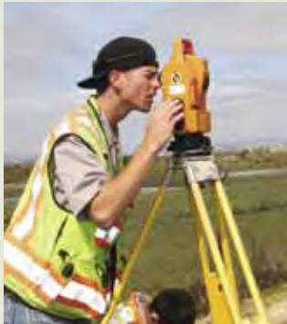
Zachary Thompson surveys the centerline station and offset distance for a set of points using an older-model total station.
