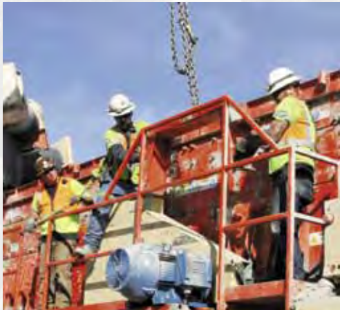
From left: Frank Fuller Jr., John Curtain and Wade Rasmussen work together to replace the drive belt on the screen box.
