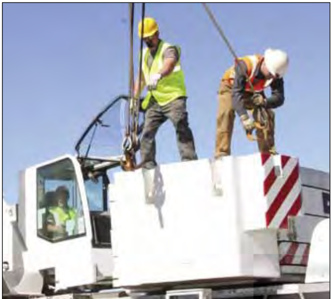
From left: Apprentices Zachary Sinclair, Josh Winters and Vince Porteous help remove the counter-weights.
