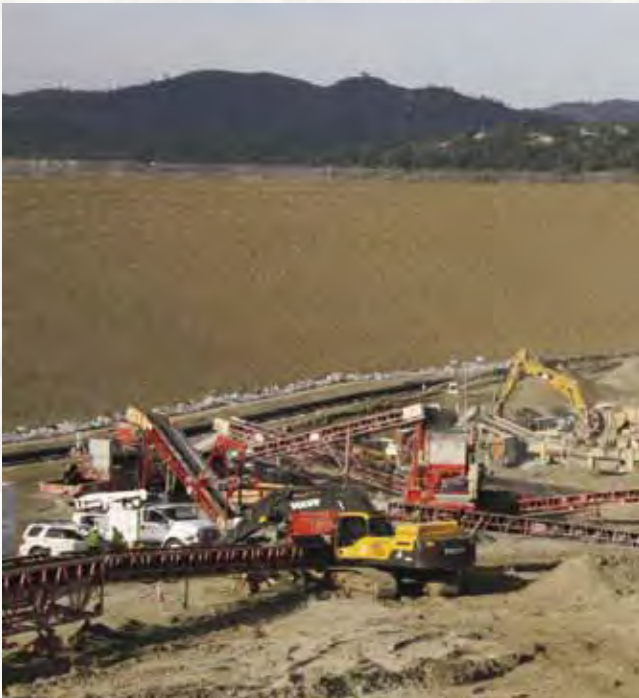
District 80 operators with Fisher Industries crush, clean and size rock th
