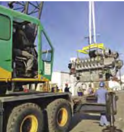
Members remove an engine from a 135-foot catamaran Vallejo ferry with only about two inches of clearance.
