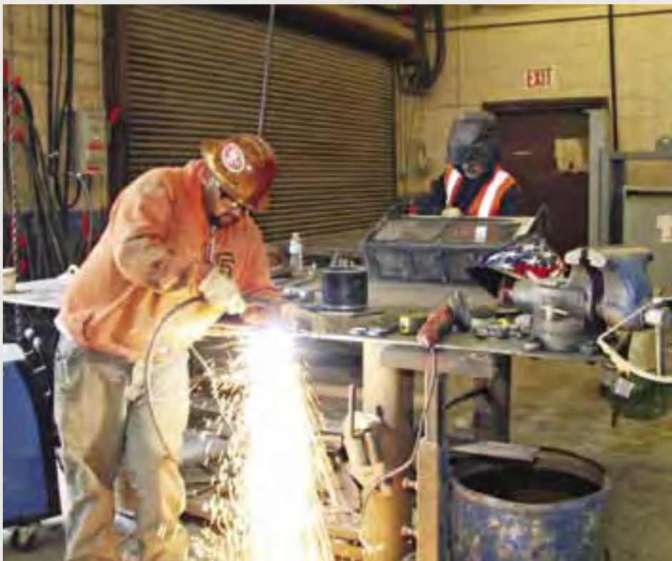
From left: Mechanic/Job Steward Andre Dias uses plasma-cutting to prepare the survey brackets for the tunnel, while Mechanic Jose Ruiz fabricates parts for the TBM.
