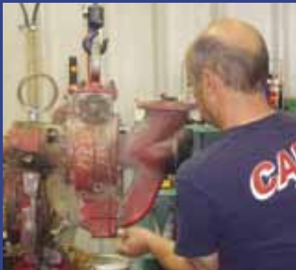
Mechanic Lewis Malotte fixes a 500-gallon-a-minute water pump.
