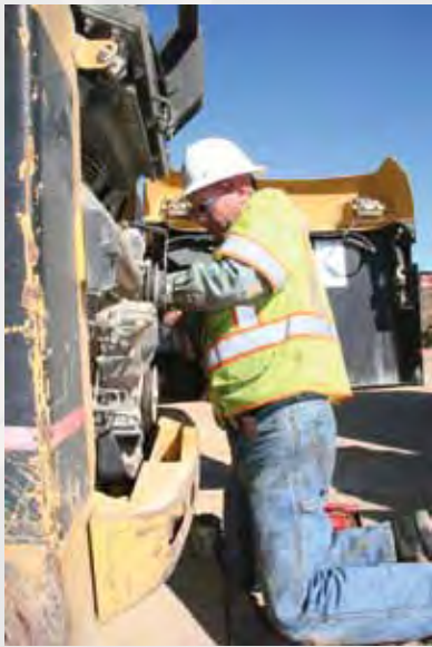
Mechanic Jamie Weeden puts an alternator and belt in a skip-loader.
