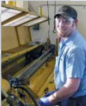
Member Michael Landon hones a cylinder in the hydraulic/machine shop.
