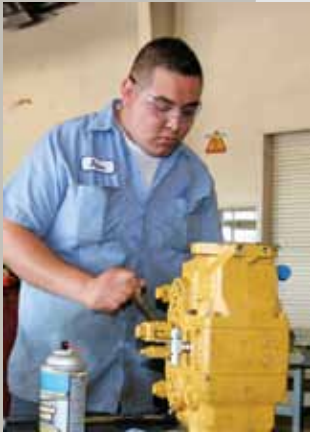
Mechanic Jesus Tinoco puts a pump back together.
