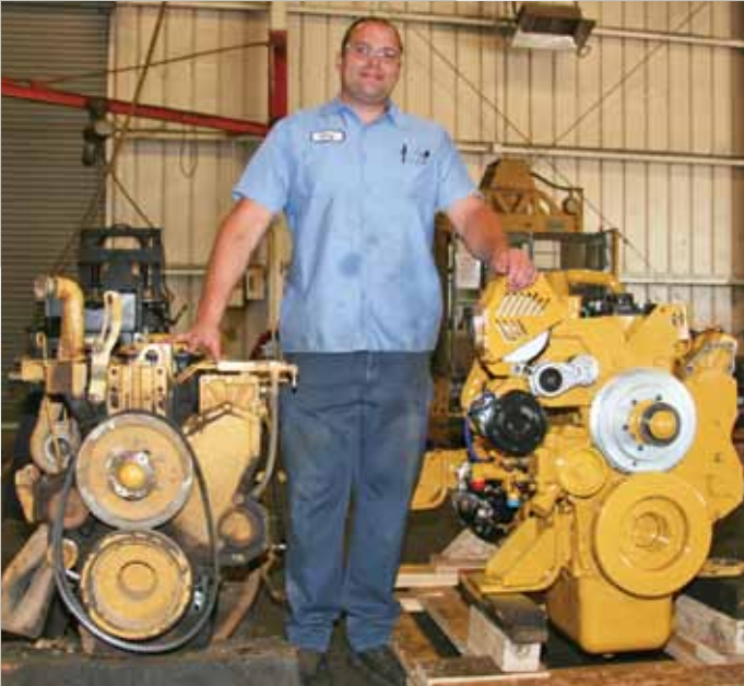
Main Shop Foreman Cory Ohlhausen stands between the new engine, right, and the old one it will replace as part of a repower of a 325 excavator.
