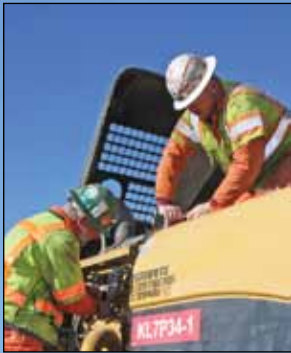
From left: Mechanics Ken Rutherford and Logan Toles take advantage of the lunch break to change filters on a 330 excavator.
