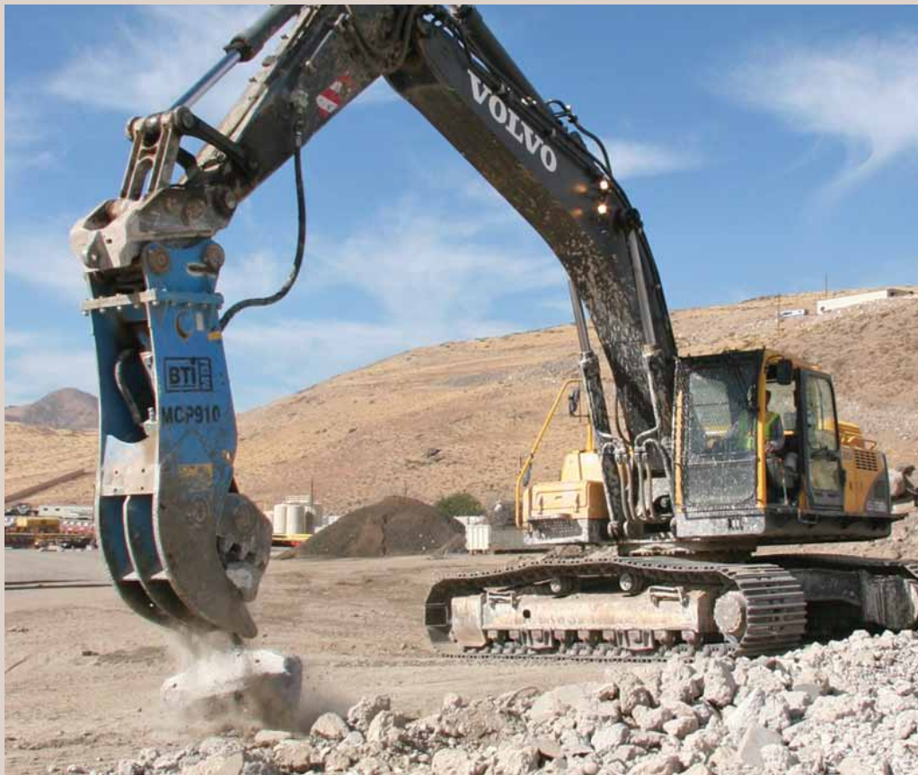
Excavator Operator Don Spears uses a jaw attachment to remove rebar from the rock pile, so it doesn't break the crusher.
