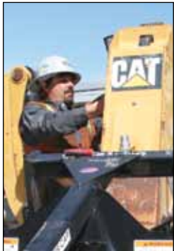
Mechanic Mike Sills fixes a starting problem on a telehandler.
