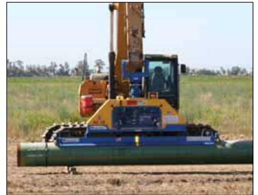
The Vacuworx attachment is made for lifting pipe on the Central Valley gas-storage project.
