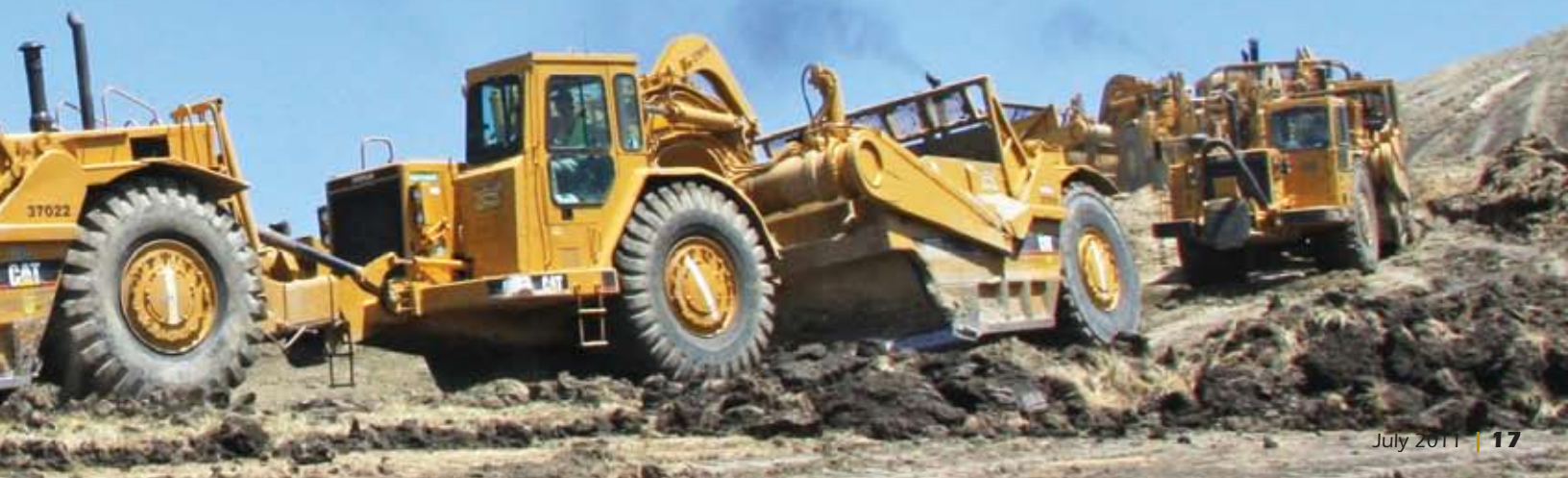
Below: Operators Jesse Espinoza and Scott Radcliff literally work together, as their 637 twin-engine push-pull scrapers hook up, filling both cans.
