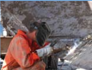
Mechanic Larry Gilley takes the cutting edge off a 657 scraper.
