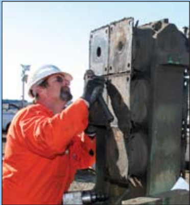
Mechanic Keith Bates replaces the rubber cushions on a vibrating hammer.
