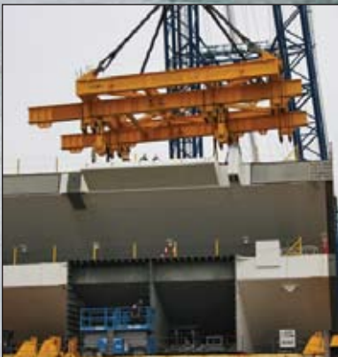
The lift bar, weighing 170 tons, and the versa bar, weighing 60 tons, are set up for the next pick.
