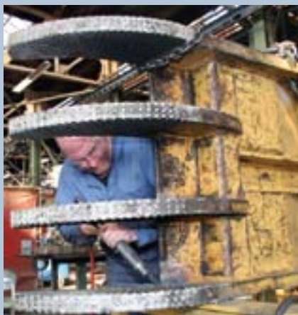
Welder Mike Paxson repairs cracks in the thumb of a 345 excavator.
