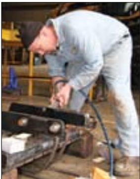
Rick Biggs replaces rollers on the lift bracket of a forklift.
