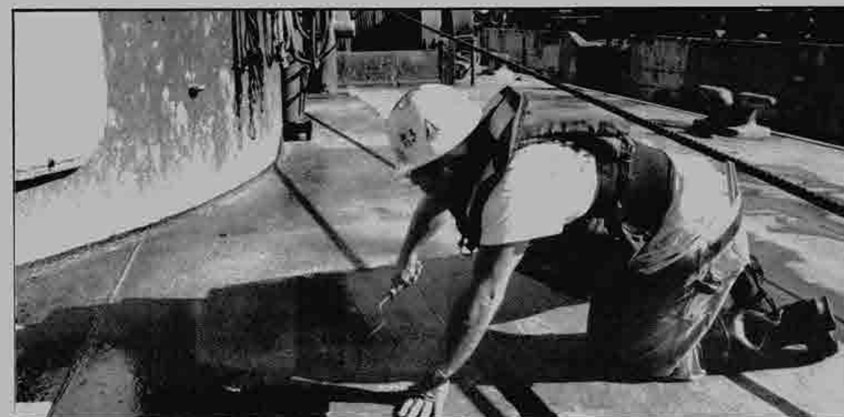
Deckhand Manuel Simas applies a coating to the deck of the Derrick Barae 24.
